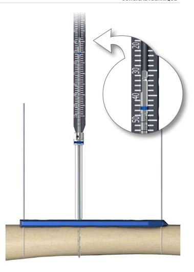
**OPTION III:** Unscrew the Guide sleeve 7.0/4.0 **[40.5705.740]** and define the screw length using the Depth measure **[40.4639.700]**.
