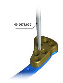
Insert Protective sleeve 9.0/7.0 **[40.5708.000]** in the desired hole of the aiming block.
